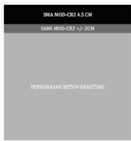
Figure 5: Pavement composition with rehabilitation strategy
